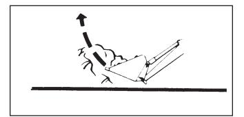
...a level bucket throughout the lifting cycle resists bucket lift and increases breakaway effort.
